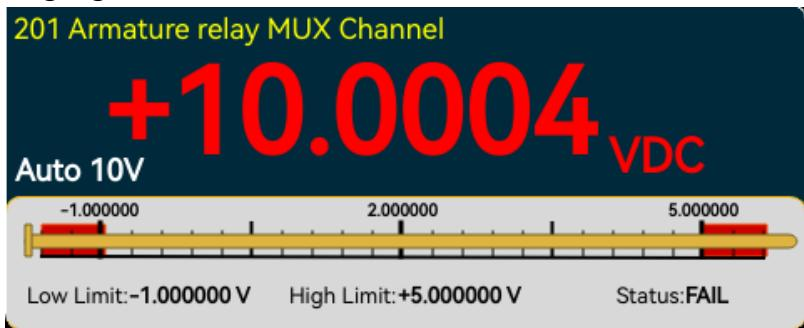
Figure 6-50 Bar meter-Alarm
