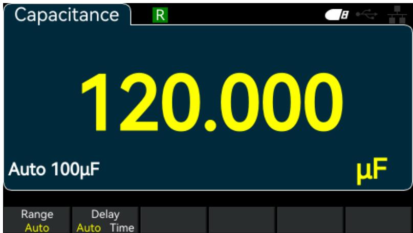
Figure 9-31 Capacitance interface
